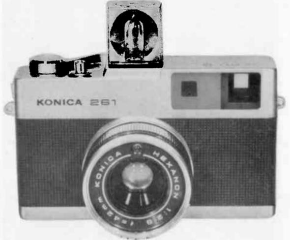
The **KONICA AUTO S 261** has a built-in flash system using an exclusive flash cube. The flash-matic system is so designed that the correct exposure is assured as the setting of the film speed **(ASA)** scale automatically determines a proper lens aperture according to the taking distance.
